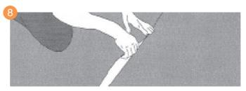
Immediately re-lay the second piece starting at the centre, press the edge into the seaming adhesive along the entire length. Any fullness of carpet should be dissipated away from the seam.
